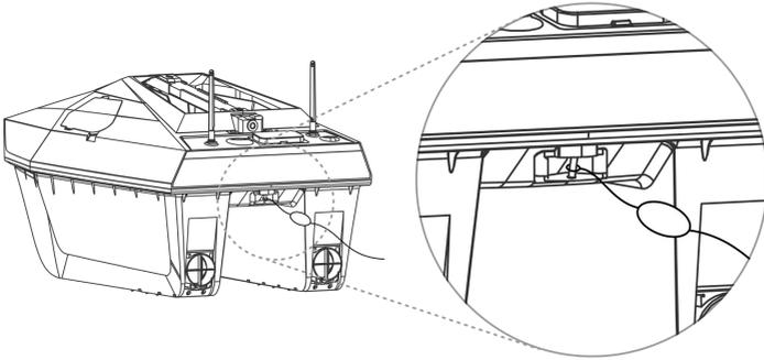
Press the button shown in **square** above to open hook release mechanism which will be open for 5 seconds and close automatically. And attach the fishing line when it is open.
