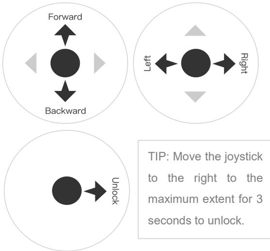
TIP: Move the joystick to the right to the maximum extent for 3 seconds to unlock.
