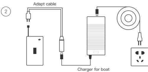
Charging the batteries separately (*please refer to **Picture2***) after taking those out of the battery compartment.
