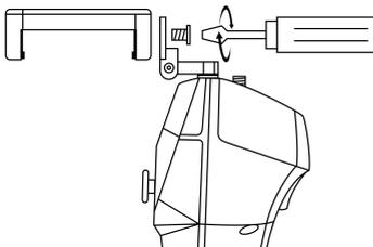
Step 2 Install the antenna
