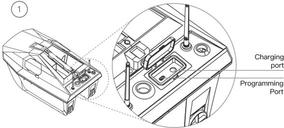
Direct charging : 5.5/2.5 DC charging port (*please refer to **Picture1***). Please note that both batteries must be inside the boat together when direct charging. It takes 4-6 hours to be fully charged; or
